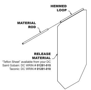
2. Hook release material rod on brackets located at the rear of the upper platen.
